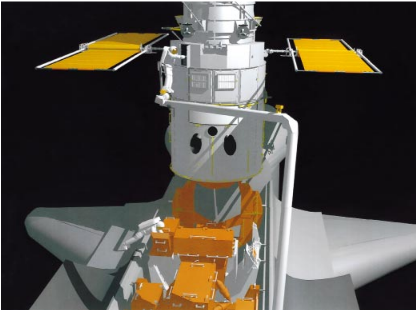
Fig. 2-12 Installation of Optical Control Electronics Enhancement Kit in Bay C
