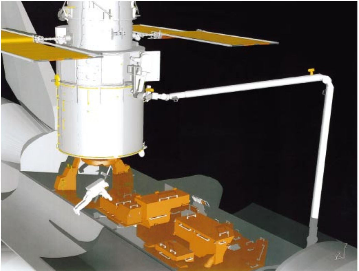
Fig. 2-11 Replacement of Engineering/Science Tape Recorder #2 in Bay 8
